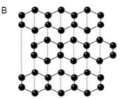
Layers of carbon atoms each bonded to 3 others. Layers weakly held together by delocalized electrons.
