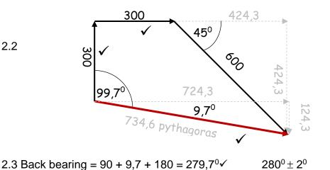
$\begin{array}{l} \text{R = 735 \pm 5m} \\ \text{bearing } 100^{0} \pm 2^{0} \end{array}$
