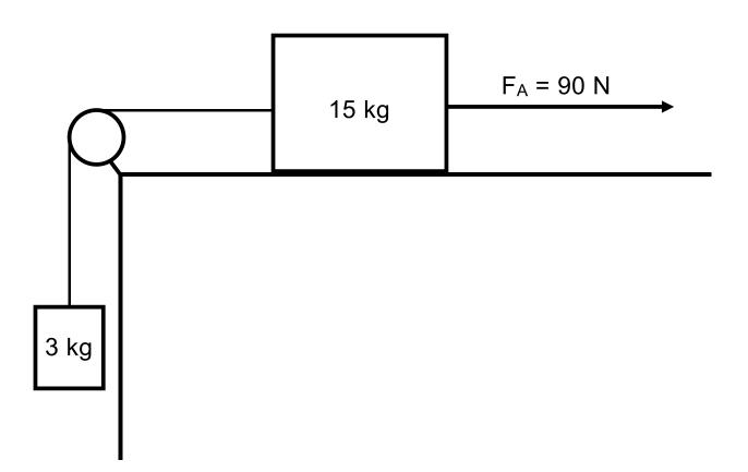
The coefficient of kinetic friction between the 15 kg block and the horizontal surface is 0,35.
