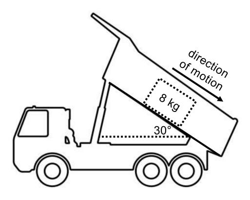
A constant kinetic frictional force of 4,4 N acts on the crate as it slides down the incline.
