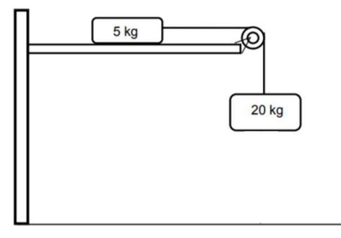
When the 5 kg mass is released, the two masses begin to move. The coefficient of kinetic friction,  $\mu_k$ , between the 5 kg mass and the horizontal surface is 0,3. Ignore the effects of air resistance.
