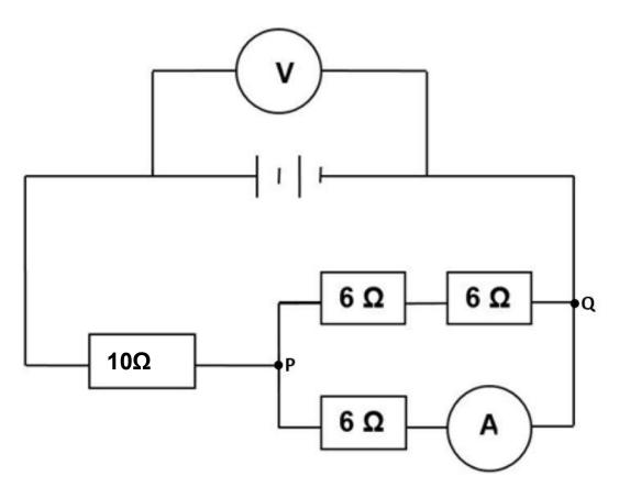
The power dissipated in the 10  $\Omega$  resistor is 0,45 W.
