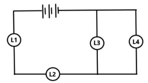
How does the brightness and potential difference of **L4** compare with the brightness and potential difference of **L1**?
