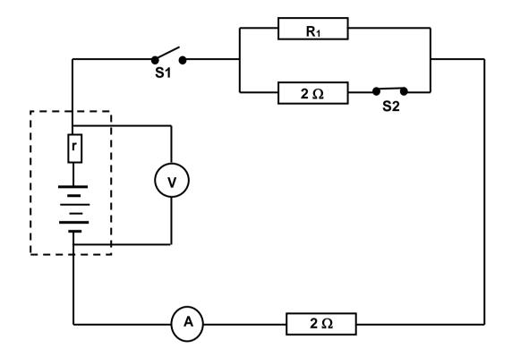
If switch  ${\bm S}_1$  is closed, the reading on the voltmeter is  ${\bm 6}, {\bm 86} \; {\bm V}$  and on the ammeter is  ${\bm 2} \; {\bm A}.$
