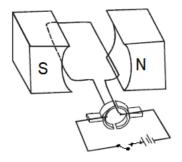
When the switch is closed, the coil rotates:
