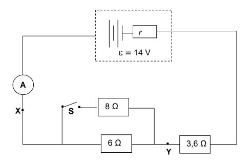
When the switch **S** is open, the ammeter reading is 1,4 A.
