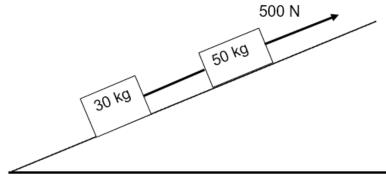
The ratio of the parallel and perpendicular components of the gravitational force on each crate is **5:3**. A force of 500 N is applied as shown on the 50 kg crate so that the crates move with an acceleration of 2 m·s<sup>-2</sup> up the incline.
